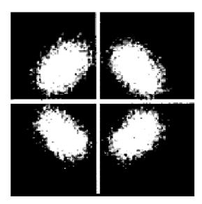
QPSK signal with phase noise (LNC)
